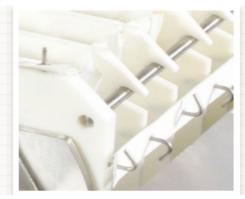
PRESSING CYCLE With a lever push, the moving platen compresses the racks together, creating juice. At the end of the pressing cycle, pull back on the lever to reopen the pressing module.
